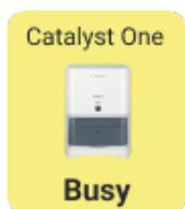
A yellow **Busy/Standby** icon indicates that the instrument is currently in use, either running sample tests or running some other process, such as quality control or standby mode.
